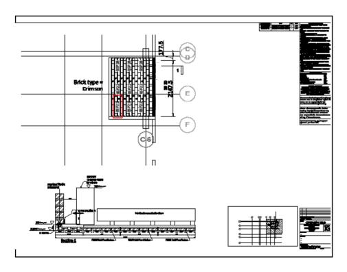
Offer up the first Brick Panel System unit at the datum point ensuring it is supported by a jig where necessary.
