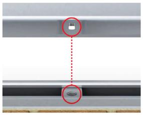
Insert spring nuts via the channel and align them to the centre of the slotted holes on the WMS system.
