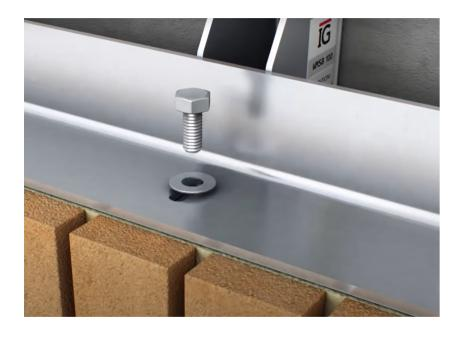
Offer up the B.O.S.S. A1 unit up to WMS and insert bolt through slotted hole on the horizontal shelf, picking up the prepositioned spring nut in the channel.
