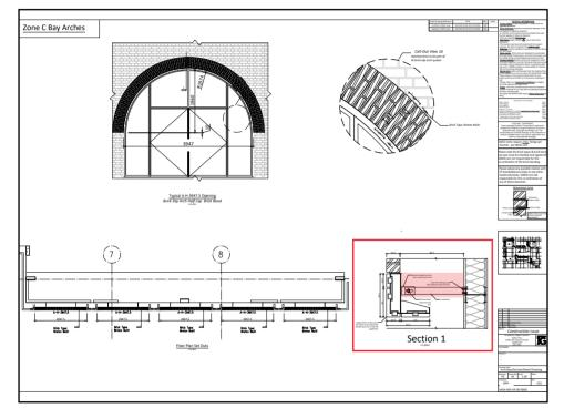
Using the Construction Issue Drawings, identify the position that the restraining brackets have to be installed (brackets supplied by IG Masonry Support).
