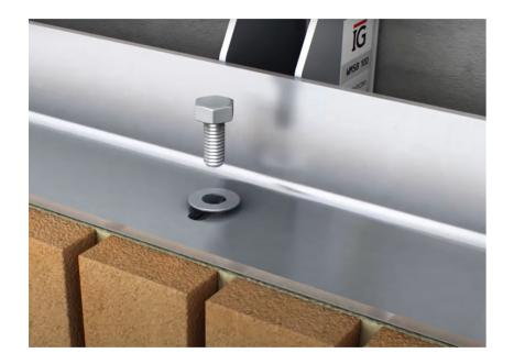
Offer up the B.O.S.S. A1 unit up to WMS and insert bolt through slotted hole on the horizontal shelf, picking up the prepositioned spring nut in the channel.
