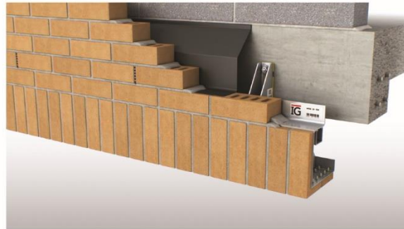
(c) Completion of surrounding brickwork
