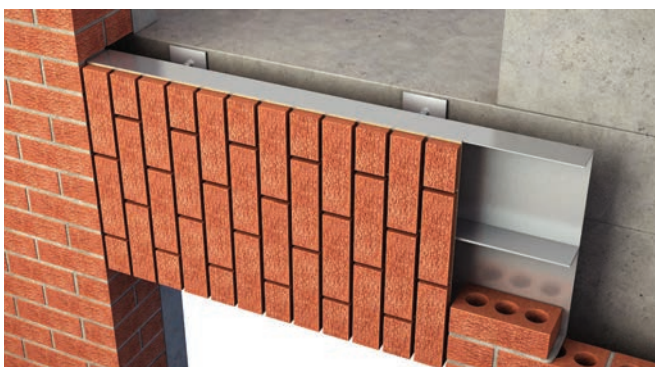
Step 1 The brick slip panel is positioned, fixed and built into the outer skin.
