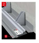
Offer up part B to the pre-installed masonry support system until it interlocks with part A.
