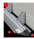
Offer up point A of the prefabricated component to the pre-installed masonry support system, keeping point B in a downward position.
