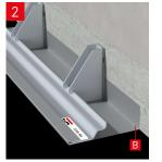
Rotate the component Align and level the until point B comes in contact with the bottom before fixing to the heel of the bracket the pre-drilled holes. and the component is horizontal in profile.
