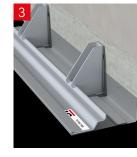
Align and level before fixing back to the substructure, utilizing the pre-drilled holes.
