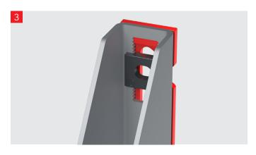
Engage the male side of the shim with the serrated section of the masonry support bracket and the lock washer, ensuring the top of the shim aligns with the top of the bracket. The serrated portion of the shim must engage with the top two teeth of the bracket's serrated section.
